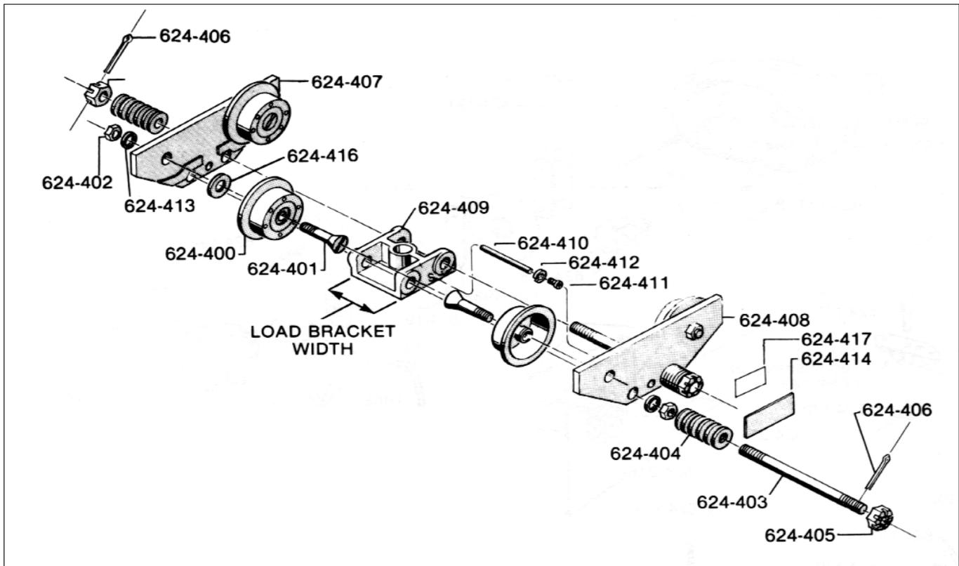
Figure 18. Series 635 Low Headroom Trolley Exploded View
