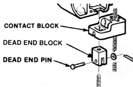
**NOTE:** Model WR is furnished with a contact block. The dead end block passes through the contact block and the contact block is supported by the dead end pin.
