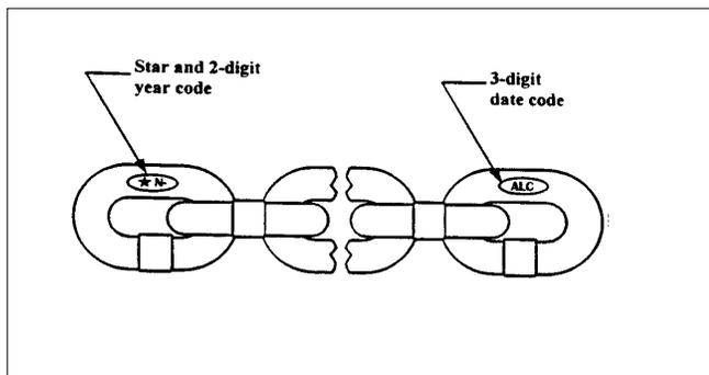
Use only CM Star (®) Grade Load Chain and CM replacement parts. Use of other chain and parts may be dangerous and voids factory warranty.
